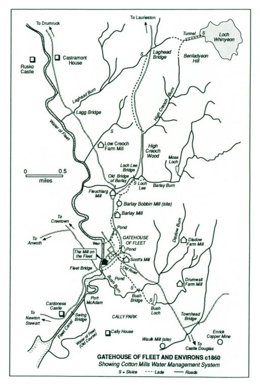
present Laurieston Road. By the bridge a sluice diverted water into a lade which ran to the west side of the present road, passing under same at a point opposite High Creoch Farm, and joining the High Creoch Burn. The combined water then flowed down through High Creoch Wood to intercept the Barlay Burn above Loch Lee Bridge. The Barlay Burn was also supplemented by water from Moss Loch, adjacent to High Barlay Farm, and its feeder streams.
